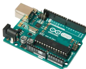
Figure 3 – UNO Arduino board
