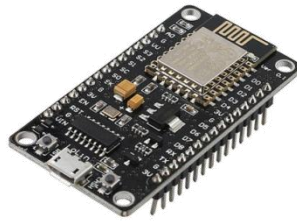
Figure 4 – NodeMcu module in combination with CH340G chip
