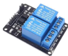
Figure 10 – Dual channel relay module
