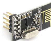
Figure 9 – NRF24L01 + wireless transmitter and receiver module
