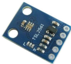
Figure 7 – TSL2561 light intensity sensor module
