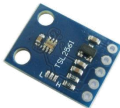
Figure 7 – TSL2561 light sensor module
