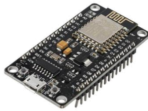
Figure 4 – NodeMcu module together with a CH340G chip
