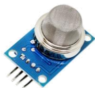
Figure 8 – MQ-135 air-quality detection sensor module
