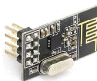
Figure 9 – NRF24L01+ wireless sender and receiver module
