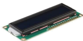
Figure 11 – Character LCD with dimensions of 16 \times 2
