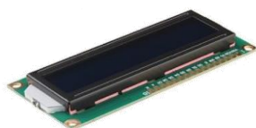
Figure 11 – LCD with 2*16 characters
