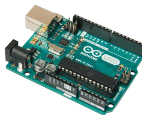
Figure 3 – Arduino UNO board
