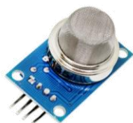
Figure 8 – MQ135 air quality sensor module
